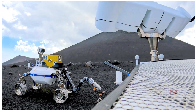
Fig. 1: Impression of an experiment on multi-robot information exchange with our two Lightweight Rover Units (LRUs) on Mt. Etna, Italy. LRU1 (in the front) selects one of the stones via its science camera and tells LRU2 (in the back) to collect it with its manipulator.
