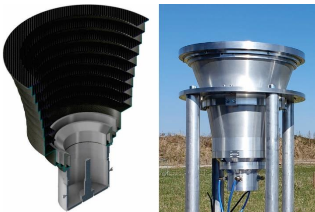
Figure 3: C-band choked Gaussian horn antenna (VeGA).
