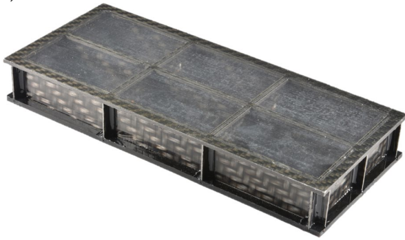
Fig. 8 Picture of the PR liner prototype without pre-tension
