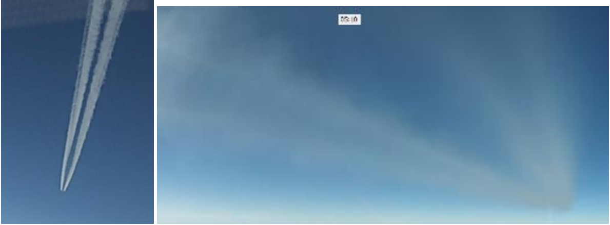
Fig. 3 A359 intercept at 5 km distance ( left ), and in the vortex pair, at 15 km distance ( right ).
