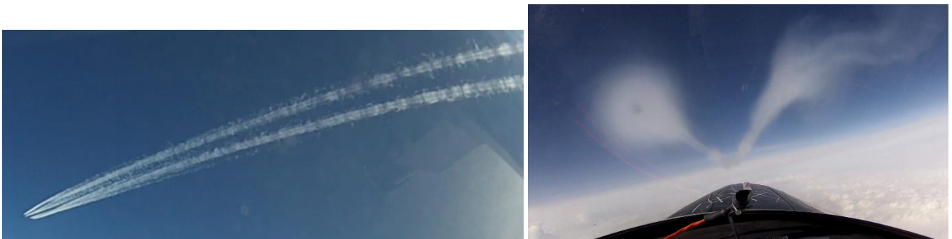
Fig. 2 A380 intercept at 3 km ( left ), apparent curvature is a camera focal length effect; at \approx 20 km ( right ), vortices in asymmetric state.
