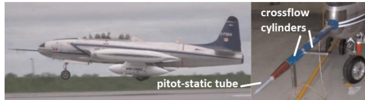
Fig. 1 NRC CT-133: underwing instrumentation pods ( left ); close-up view ( right ) shows the nose boom with pitot-static tube, and crossflow cylinders for flow angle measurement.
