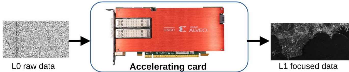
Overview of SAR focusing flow, adapted from [2]
