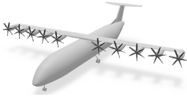
Figure 4.6: ESBEF-CP1: a hydrogen-powered concept aircraft developed by the German Aerospace Center (DLR). Reproduced from Bielsky et al. (2023).
