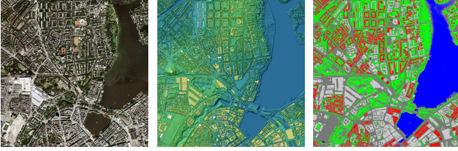
Fig. 1. Test region Hamburg, 3 \times 3 \text{ km}^2 , left: Ortho image from the WorldView-4-scene, center: derived DSM, right: derived classification (blue: water, light-green: grass, dark-green: tree, red: adobe roof tiles, light-gray: concrete on flat roofs, dark-grey: asphalt/road, yellow: bare soil).
