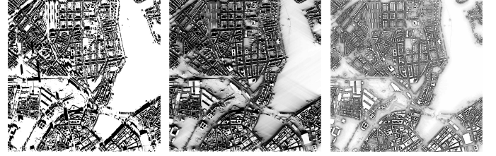
Fig. 2. Same test region Hamburg, 3 \times 3 \text{ km}^2 , left: shadow 2018-10-05 at 10:30 UTC, center: mean of all shadows of the day, right: skyview.
