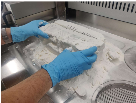
(a) Powder block containing all the printed parts.
