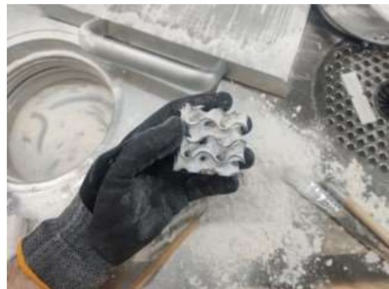
(b) Cleanup of the PA12 powder from a gyroid cube.
