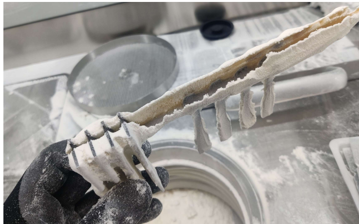
Figure 6.1: A first PA12 print fail caused by the recoater dragging one of the parts.
