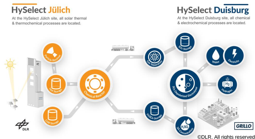
Fig. 1: Scheme of the HyS. On the left side, the SAS is performed utilizing solar energy in Jülich; on the right side, the SDE is performed on a second site, Duisburg (both Germany)
