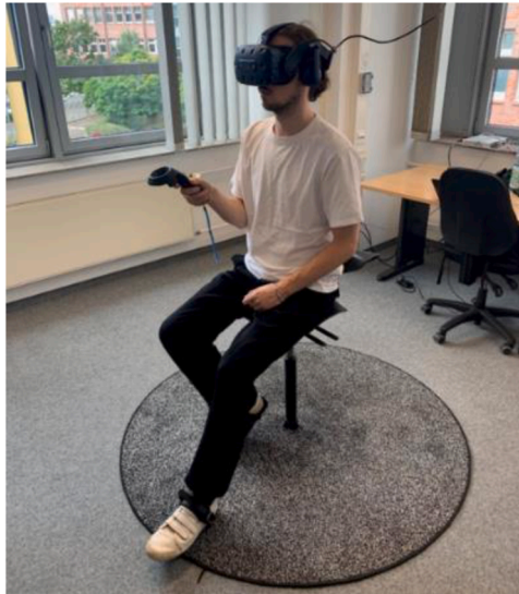
Fig. 4. Study participant wearing the VR headset to see, and sitting on the 360° rotatable chair and wearing the Cybershoes to move in the VR environment.
