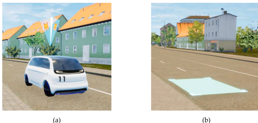
Fig. 9. vStop HMI information elements to identify the shuttle. (a) diamond shaped shuttle highlighter, (b) stopping position highlighter.
