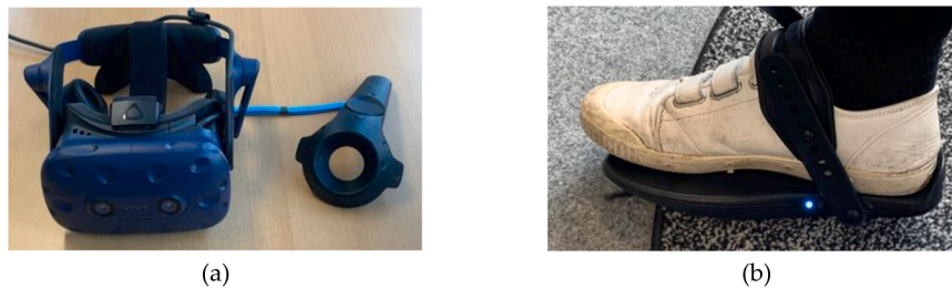
Fig. 3. Wearable VR equipment used in the user study. (a) Vive Pro HMD with controller, (b) strapped Cybershoes.
