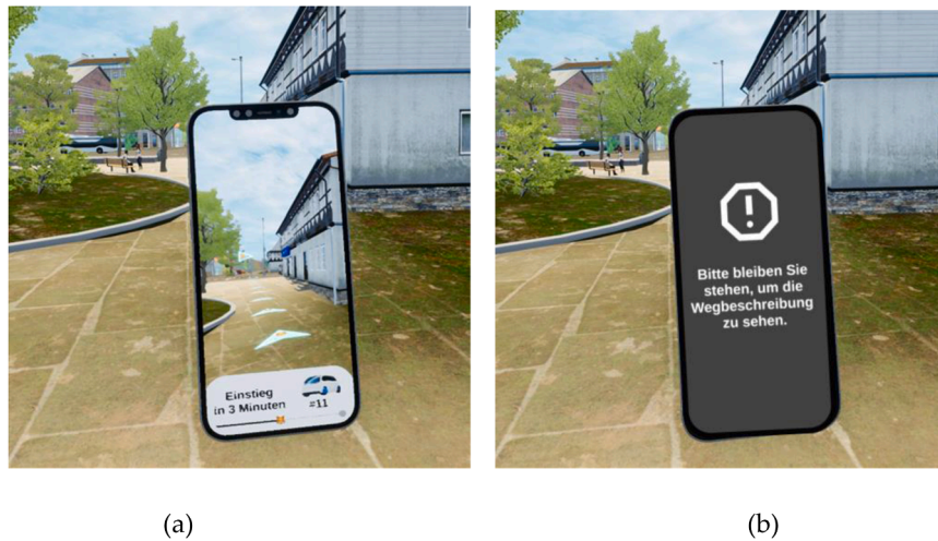
Fig. 8. Overview of the HMI variants during the navigation task. (a) View of group A that used the HMI without information restriction. (b) View of group B that used the HMI with the treatment of information restriction when walking.
