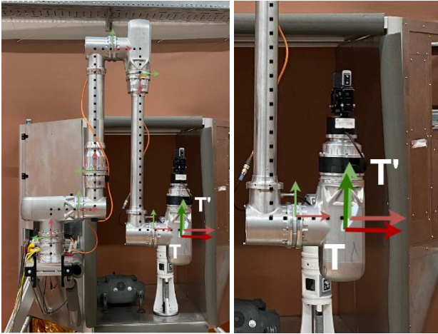
Fig. 5. TINA arm bending due to gravity.
