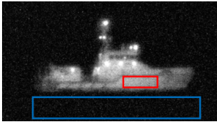
Fig. 8. ROIs for SNR and contrast calculation; red rectangle inside of ship hull (high intensity); blue rectangle outside of ship (low intensity)
