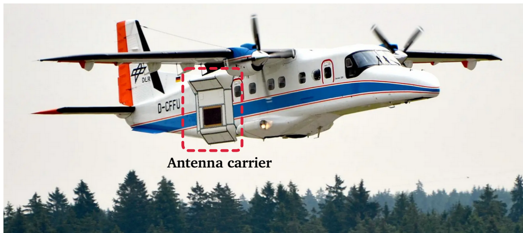
Figure 2.11.: DLR's research aircraft Do-228-212 D-CFFU. The antenna carrier is installed sideways on the aircraft.
