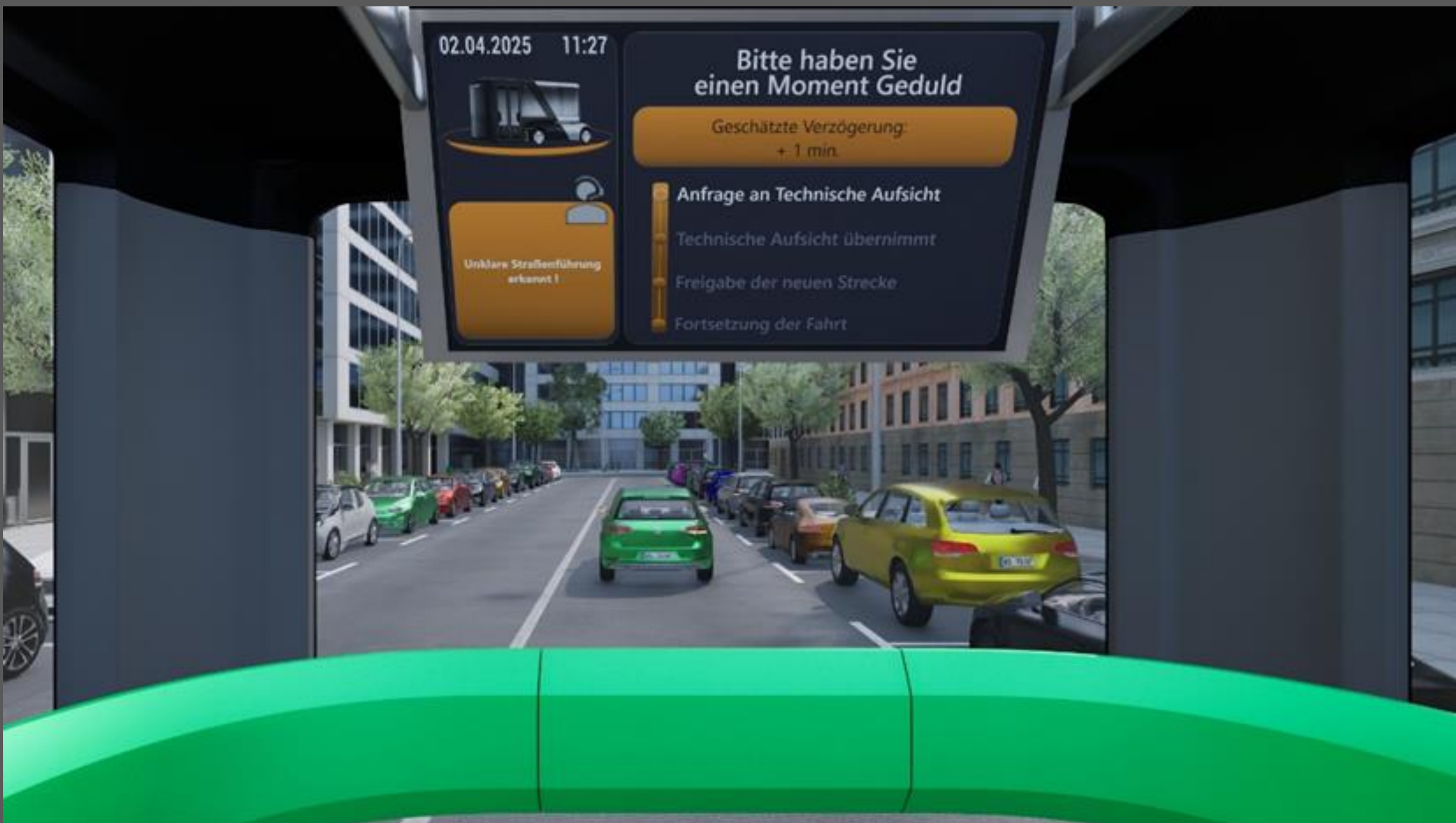
Figure 1: Text-based HMI displaying information on the MRM.
