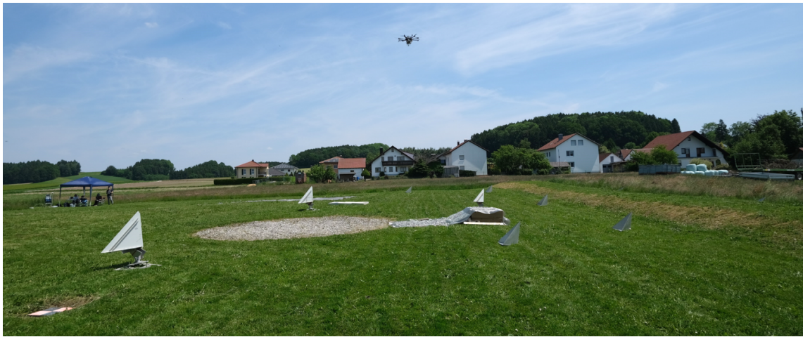
Figure 6.5: Photograph of the test site including the corner reflectors and the drone flying during an acquisition.
