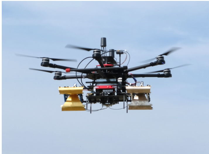
Figure 6.4: Photograph of the UAV with the radar system onboard.
