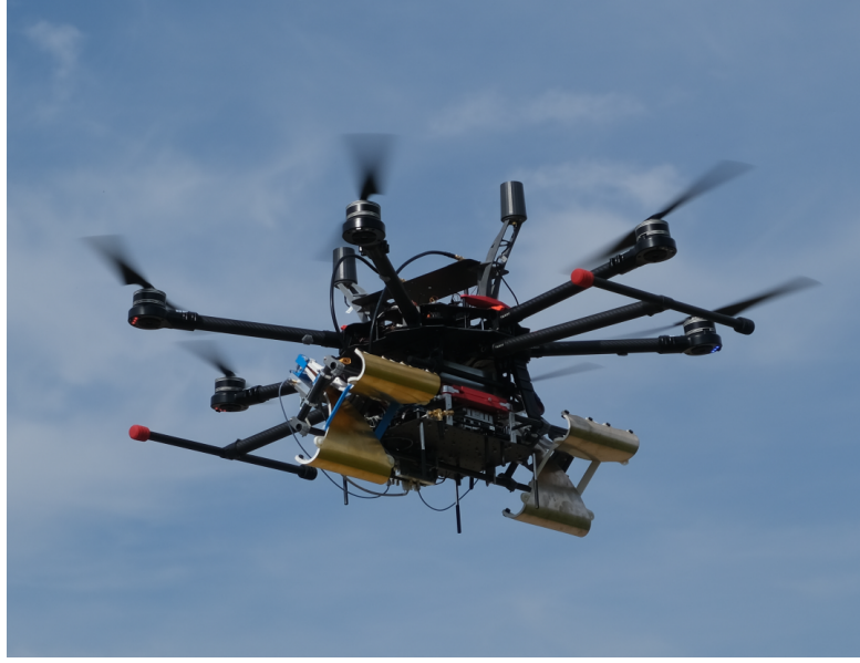
Figure 3.1: Photograph of the drone employed in this thesis with the radar system onboard during a flight.
