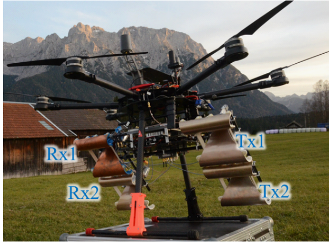
Figure 6.22: Photo of the drone and radar system employed in the experiment. The transmit and receive antennas are indicated.
