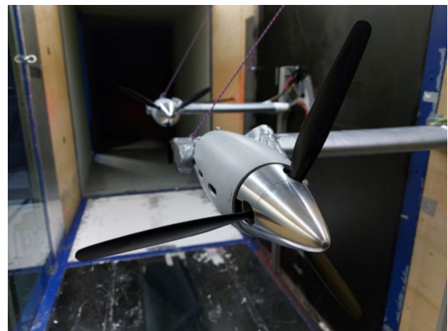
Fig. 3 Set up of tandem propellers in cruise flight conditions at the S. De Ponte wind tunnel [14]
