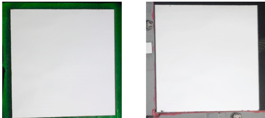
Fig. 11. Photographic images of the whole sample surfaces. Left: RLA4R sample after 6000 h of the DH test; Right: RLA3 sample after 6000 h of the COND test.
