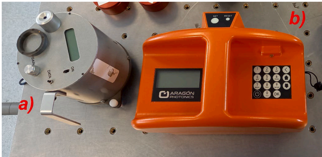
Fig. 3. Reflectometer devices used for field measurements, a) D&S-15R on the left and b) Condor by Zepren on the right.
