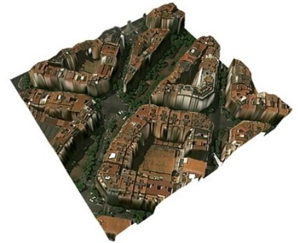
3D reconstruction of a satellite image using the predicted height by the proposed FusedSeg-HE model
