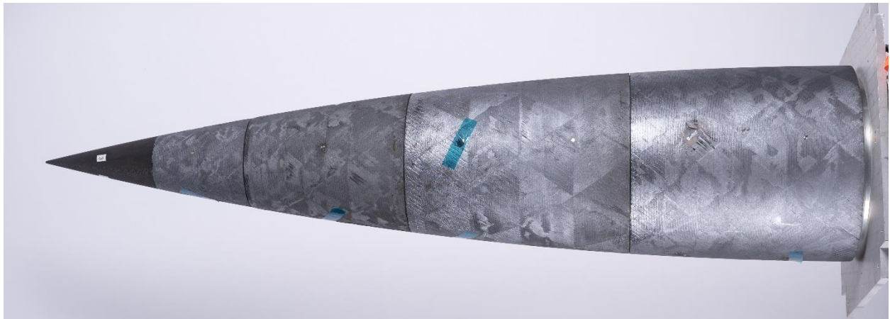
Figure 4: CMC forebody of STORT.
