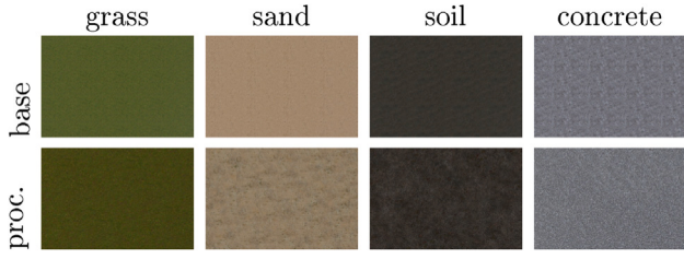
Fig. 3. Comparison of the four different ground textures. Top row: simple textures based on repeating image patches. Bottom row: procedural, randomized ground textures with 3D effects.
