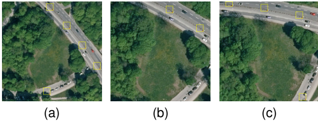
Fig. 5: Shadow simulation via image rotation: (a) Original patch, (b) Patch rotated by 20^\circ , (c) Patch rotated by 40^\circ .
