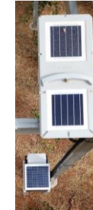
Side-by-side reference cells (soiled vs clean)
