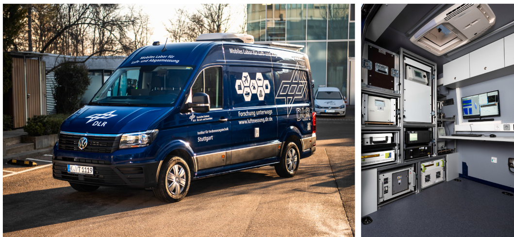
Fig. 1. The DLR mobile lab for the measurement of particles and combustion gases. On the left side: View of the vehicle from the outside. On the right side: View of the mobile laboratory with built-in measuring devices.
