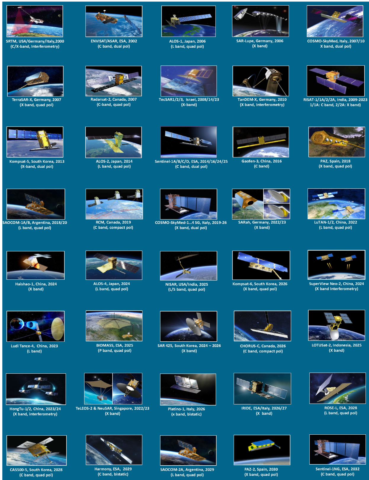
Fig. 7. Overview of past, current, and planned full-fledged spaceborne SAR systems (2000 onward, sources: https://www.eoportal.org/ ; https://space.oscar.wmo.int/ ; and https://space.skyrocket.de ). The dates indicate the launch year of the satellite or satellite series. NewSpace SAR systems are shown in Fig. 13 and described in Section IV.
