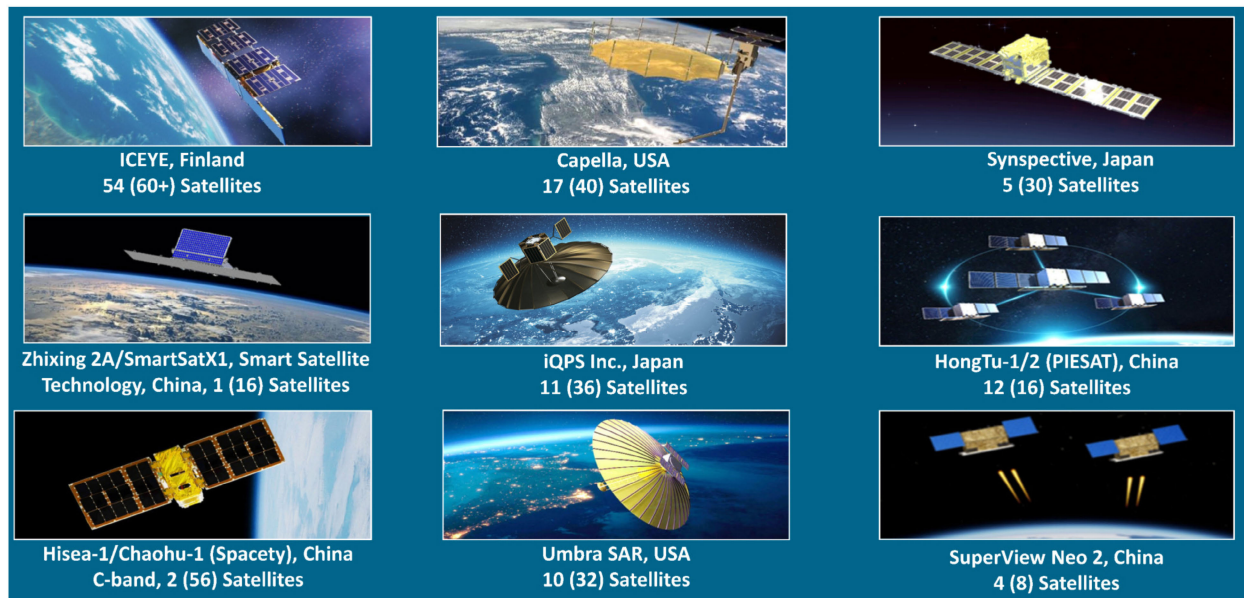
Fig. 13. Examples of NewSpace SAR systems with the respective number of satellites launched as well as planned launches (in brackets) as of October 15, 2025 [101], [102]. ICEYE, Capella, and Umbra are leading the commercialization of NewSpace SAR imagery, followed by iQPS and Synspective. Typical weights of NewSpace SAR satellites are in the range of 85–250 kg, much less than full-fledged SAR systems, weighing approximately 1–2.5 ton, due to their much greater imaging capacity and coverage.
