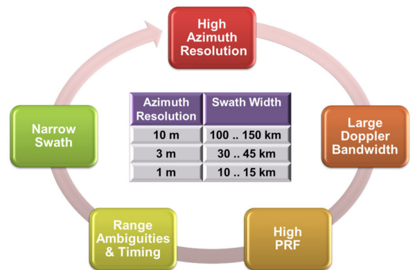
Fig. 4. SAR system design dilemma for conventional SAR systems, showing the main tradeoff between swath width and azimuth resolution. The table depicts typical tradeoffs between azimuth resolution and swath width for a spaceborne SAR system.
