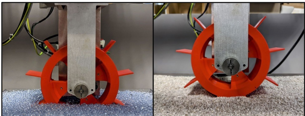
Fig. 8 Examples of wheel sinkage into different types of surface materials: (left) glass beads and (right) quartz sand. In both examples the load applied to the wheel is the same but the sinkage is different
