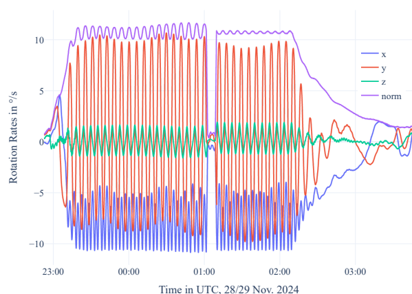
Fig. 12: Rotation rates during the spin-up and detumbling test.
