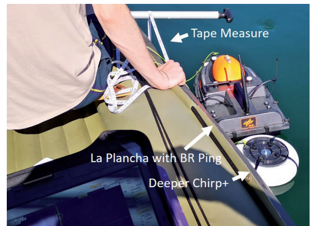
Fig. 9 - Validation of two sonars (Blue Robotics Ping and Deeper Chirp+) against a tape measure at 62 points at different depths
