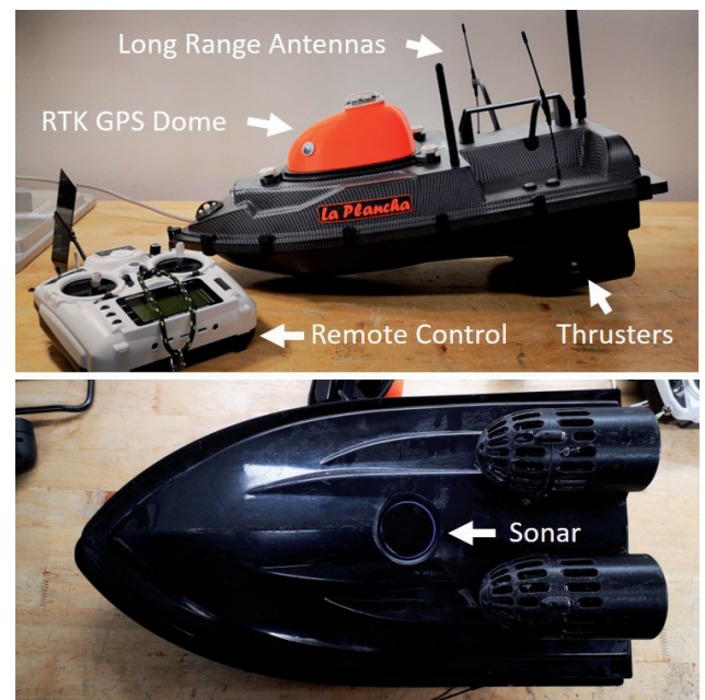
Fig. 2 - The ultra-compact bathymetric survey vehicle "La Plancha" of DLR
