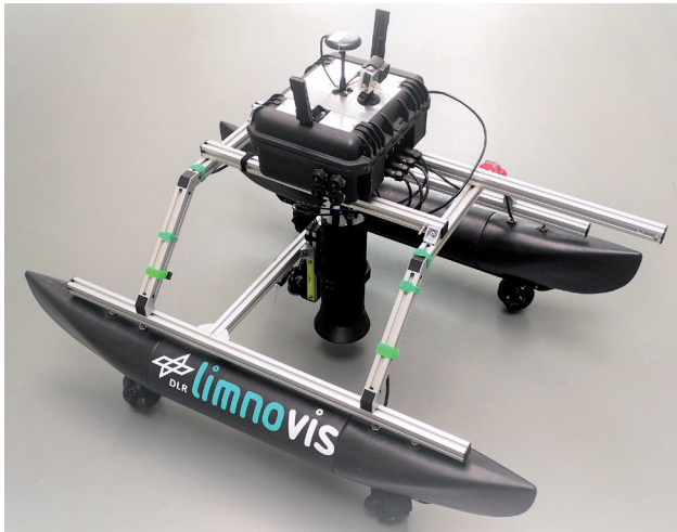
Fig. 4 - USV LimnoVIS of DLR, equipped with downward facing underwater camera in a watertight housing
