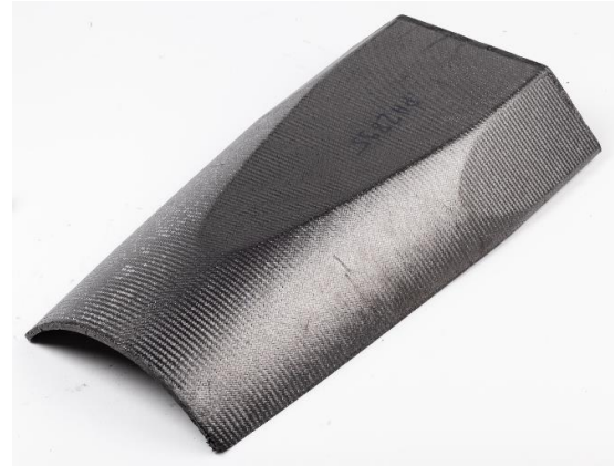
Figure 13 Segment C part in C/C condition.
