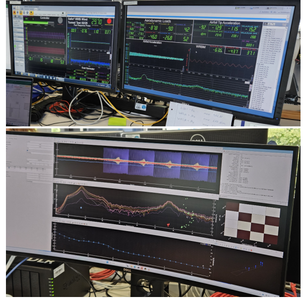
FIG 4. Images of the data monitoring setup used during the experimental tests. Top: Sensor signals of the wing demonstrator via Dewesoft. Bottom: Online operational modal analysis.
