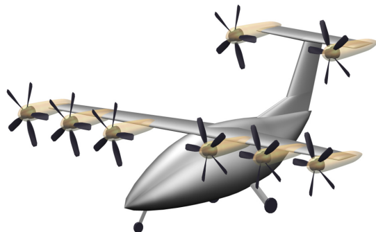
FIG. 1. Visualization of the electrically powered tilt-rotor vehicle.
