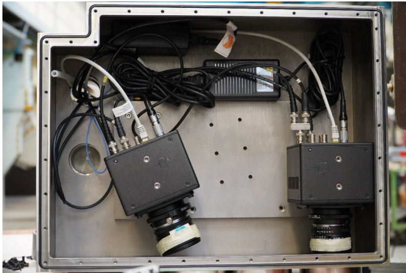
Figure 7: DIC system box and cameras (flow from right)
