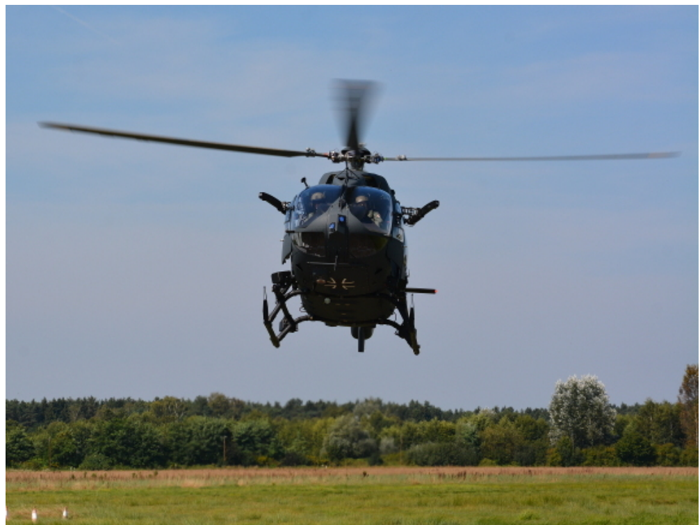
Figure 1. H145-LUH-SOF in the configuration used during the flight experiments, with left and right fast rope beams extended.
