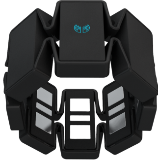
Figure 3.1: Myo Armband from Thalmic Labs with 8 sensor modules and 200 Hz sample rate [3].
