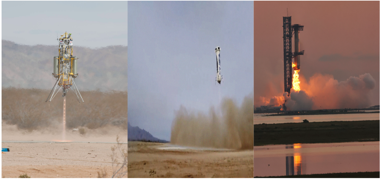
Figure 1.1: Examples of VTVL vehicles. From the left: (a) Xombie demonstrates the G-FOLD algorithm (2013). (b) Blue Origin’s New Shepard first vertical landing (2015). (c) SpaceX’s Super Heavy booster performs the first successful catch landing with the Mechazilla arms (2024).
