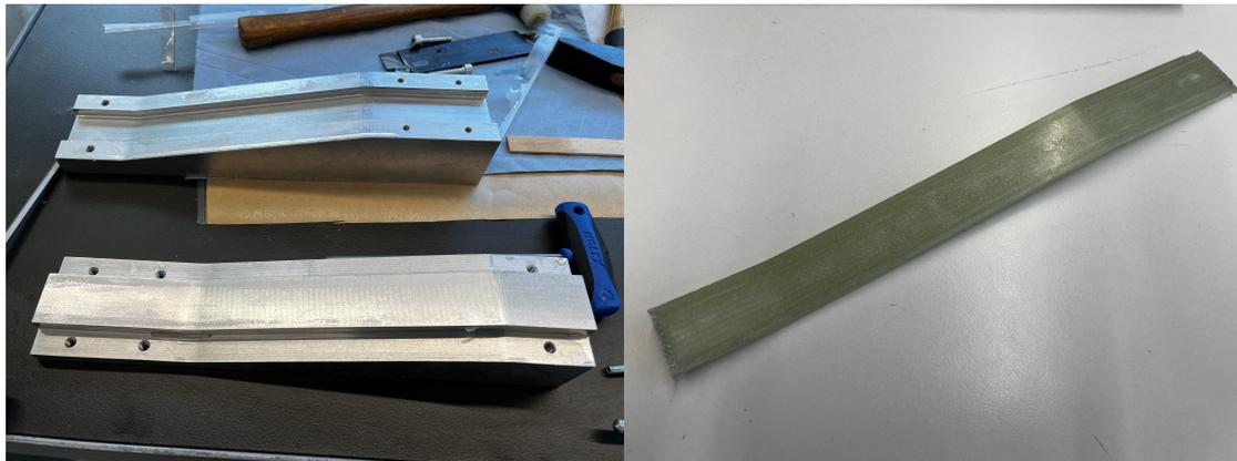
(a) Mold for beam manufacturing.
