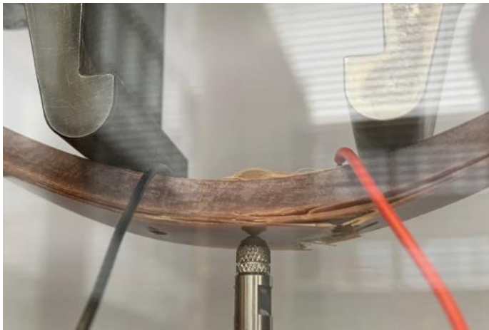
FIGURE 12: CLOSE-UP OF A FOUR-POINT BENDING TEST UNDER LOAD. THE FORCE APPLICATION ELEMENTS ARE AT THE TOP OF THE PICTURE. THE SPECIMEN IS LOCATED SHORTLY AFTER THE SPECIMEN BREAK. THE DISPLACEMENT WAS MEASURED USING AN INDUCTIVE DISPLACEMENT TRANSDUCER (PIN IN THE LOWER PART OF THE IMAGE).
