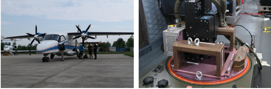
(a) DLR Research aircraft - (Dornier) DO 228-212. (b) HySpex sensor system onboard DO 228-212.
