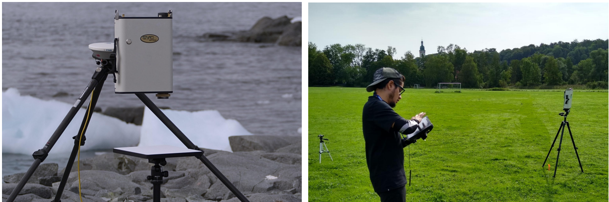
(a) Spectra Vista Corporation (SVC) spectrometer performing the measurement of a reference panel (white square below). The objective is to characterize the incoming solar irradiance, already filtered by the atmosphere. Image credit: Spectravista.
