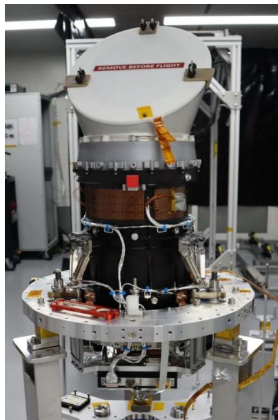
Figure 1. Picture of camera FM22 at CSL after integration of the TOU with its analogue chain (FPA+FEE),
