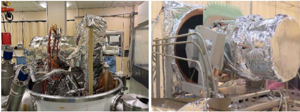
Figure 3. Picture of an FM camera installed on the hexapod inside its thermal environment box before closure of the TVAC chamber at IAS on the left, and another one in the gimbal at INTA on the picture on the right. SRON setup not shown for better figure visibility.
