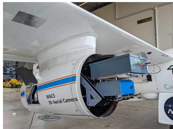
Fig. 1. The wingpod with the VHF receiver.
