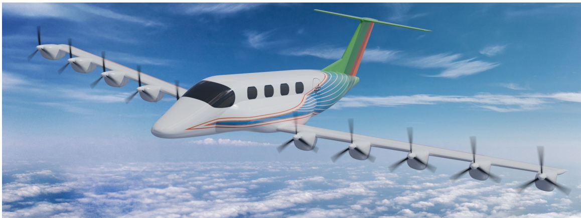
Figure 1: Concept of the Hydrogen Powered D-LIGHT+ Commuter Aircraft with Distributed Electric Propulsion
