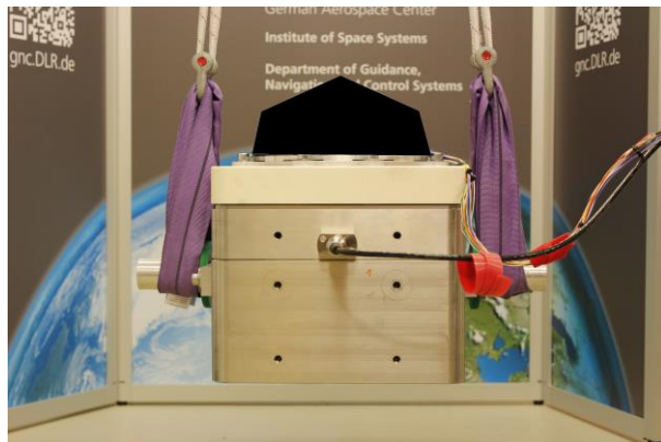
Figure 2: Suspended setup (Setup-A) in an upright position, with a dynamometer mounted on top of the seismic mass (grey) fixed with slings to elastic ropes. The reaction-wheel (black) is mounted on the top of the dynamometers ceramic plate (white).
