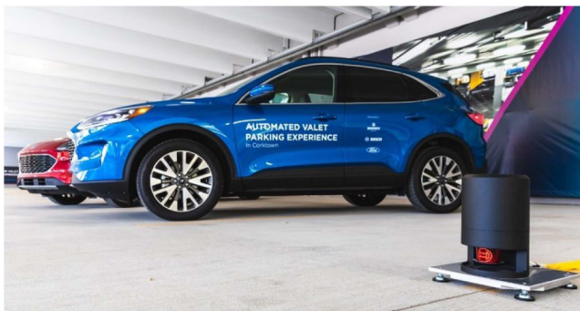
FIGURE 3. Ford Escape test vehicle guided by Bosch smart infrastructure sensors through Bedrock's Assembly Garage in Detroit [20].
