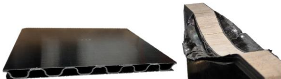
Figure 4: Left: Corrugated core; Right: Balsa wood core
