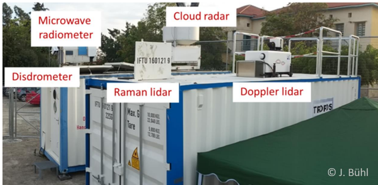
Figure 1 The measurement systems of LACROS. Different measurement systems are used to measure aerosol (Raman lidar), cloud particles (cloud radar), air motions (Doppler lidar), rain (disdrometer) and water vapor (microwave radiometer).
