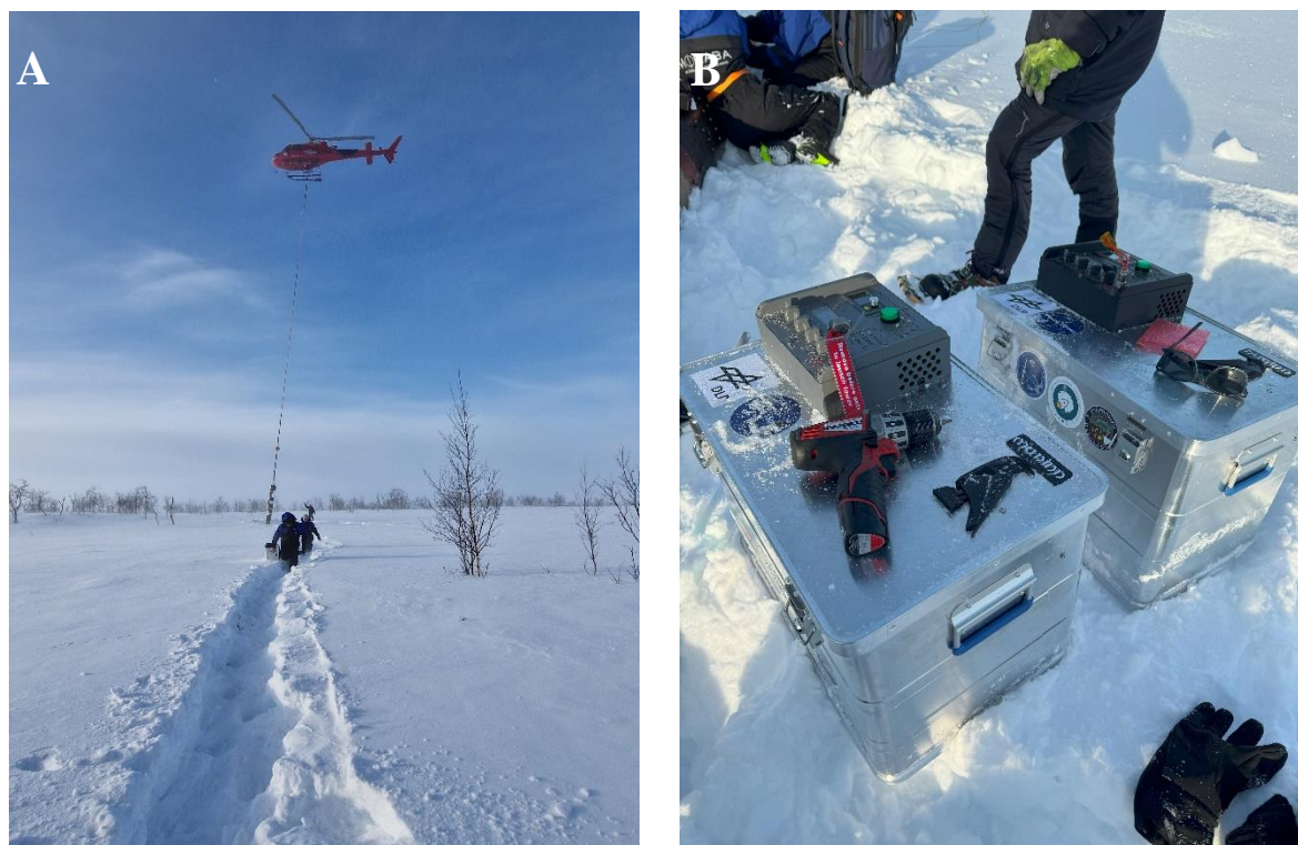
Figure 2. Transport incubators used to recover the rocket payload during the MAPHEUS-14 sounding rocket campaign. The incubators were delivered to the remote landing site by helicopter and subsequently transported through deep snow to retrieve and preserve the experimental modules under controlled conditions (A). Operation under extreme conditions in the northern Swedish tundra. After removing the experiment modules from the payload, they are recovered on-site and powered by the internal electrical system of the transport incubators. The return transport is conducted under controlled conditions within the incubators, ensuring protection during helicopter transit (B).
