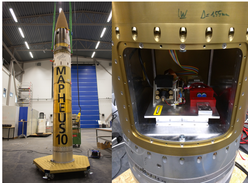
Figure 5. (left) MAPHEUS-10 payload (MExA container labeled with the number 10); (right) apex Mk.2 SCP, apex Mk.3 SES, and Trichoscope mounted on MExA integrated into the payload container.
