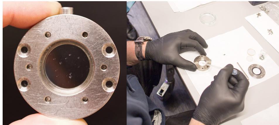
Figure 6. (left): stainless steel glass cuvette for use under vacuum conditions in space. Formerly used for experiments with Paramecium [23]. In the window, Trichoplax adhaerens animals are visible as white spots. Diameter of the glass window is 22 mm. (right): preparation of cuvette before launch.
