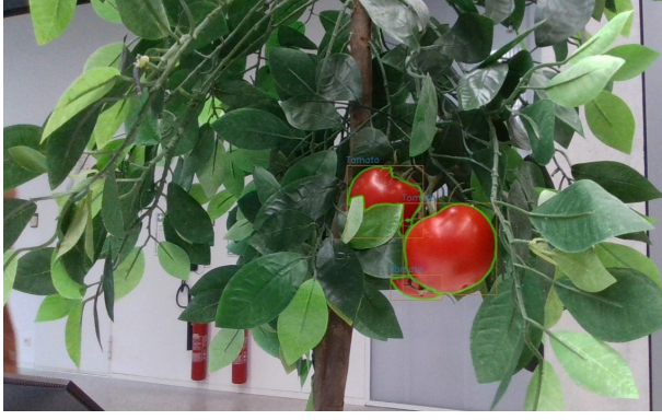
Fig. 7: A test identification of a cluster of tomatoes on the vine. Three tomatoes are in full or partial view of the camera. In this case, all three are correctly identified, as indicated by the respective masks and labels.
