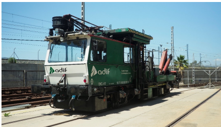
(a) ADIF maintenance train used for GNSS field data collection in Málaga, Spain.
