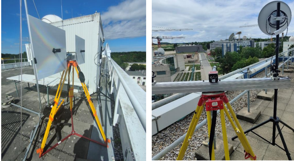
Figure 39: Test setup. Test Target at IKN (Left) and Transmitter at GSOC (Right)
